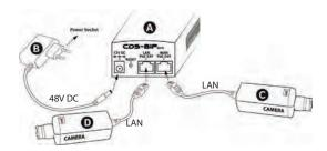
**Option 3 -** Power radio module and a camera with Switch PoE48V via an additional converter PoER-24 (option with an additional CAMSAT module PoER-24, PoER-24h).
