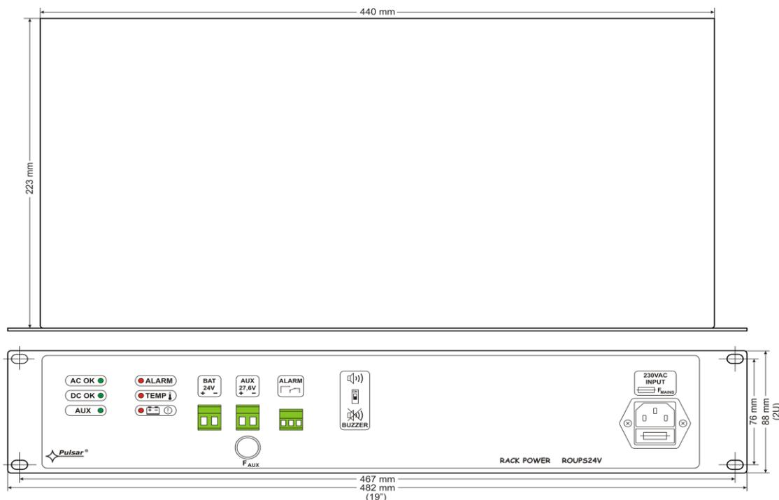
Fig.3. The view of the PSU.
