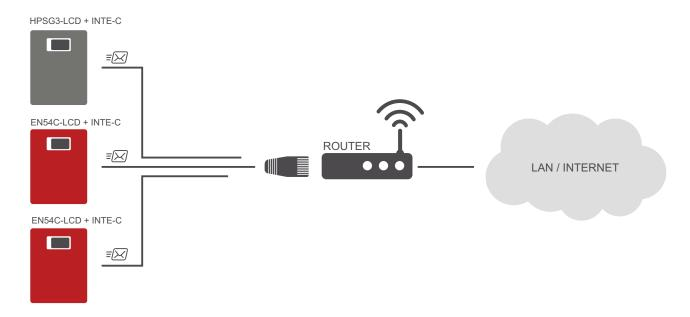
The network topology is based on the Ethernet switch (e.g. switch, router) to which subsequent PSUs with INTE-C interfaces are connected. Each interface has a static IP address. The communication between a PC and an end PSU takes place through entering the IP address of the interface.
