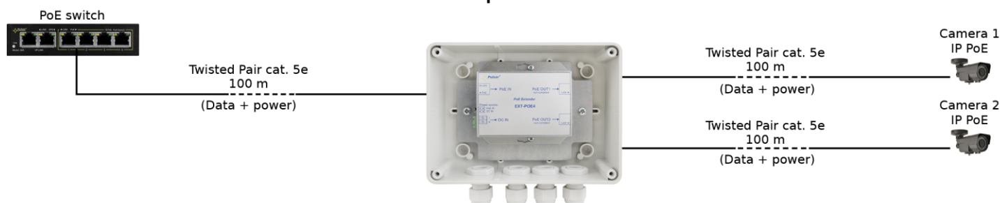
Connection of two IP PoE cameras and extension of the range for another 100m
