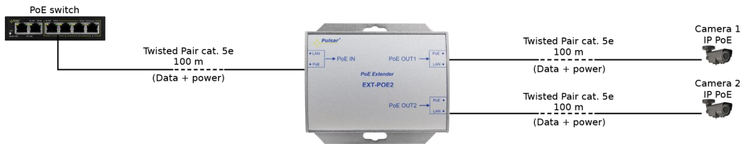
Connection of two IP PoE cameras and extension of the range for another 100m
