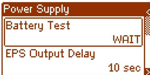
Fig. 27. Temporary battery test blockade.
