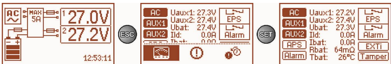
Fig. 17. LCD panel – PSU parameters.
