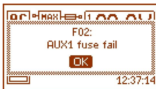
Fig. 18. Message indicating blown fuse at AUX1 output.
