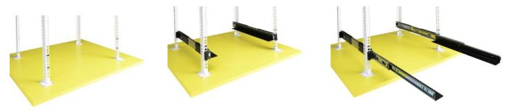
**3.2.** Place the ARAD enclosure onto the slid-out ARAS rails. Next, bolt it from the inside with M4 screws (included). The enclosure is to be fixed to the front part of the RACK rails with four 4xM6 screws.
