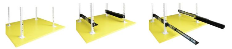
**3.2.** Place the ARAD enclosure onto the slid-out ARAS rails. Next, bolt it from the inside with 4xM4 screws (included). The enclosure is to be fixed to the front part of the RACK rails with four M6 screws.
