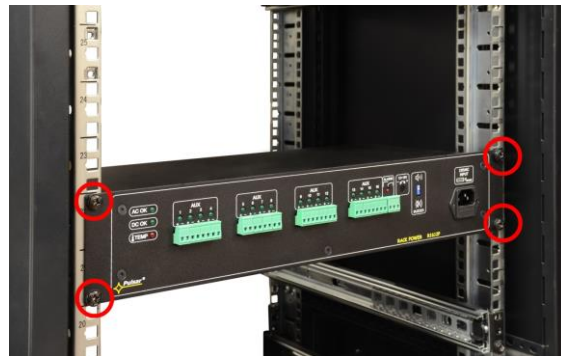
- Secure the enclosure with 4xM6 screws
