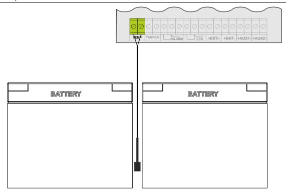
Fig. 13. Mounting of the temperature sensor.
