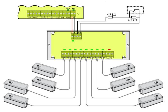
Fig. 12. Example of connection of the EN54C-LS8 sequential module with actuators with return spring.
