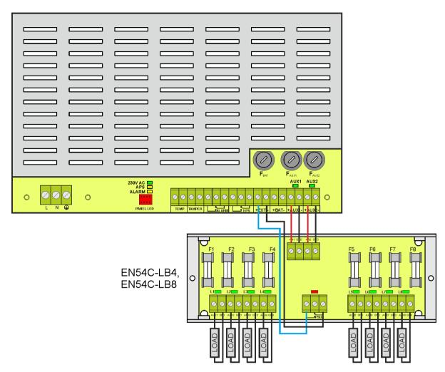
Fig. 10. Example of a connection with the fuse module EN54C-LB8.
