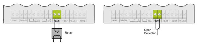
Fig. 9. Connections to the EXTi input.
