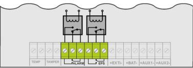
Fig. 5. Electrical diagram of relay outputs.
