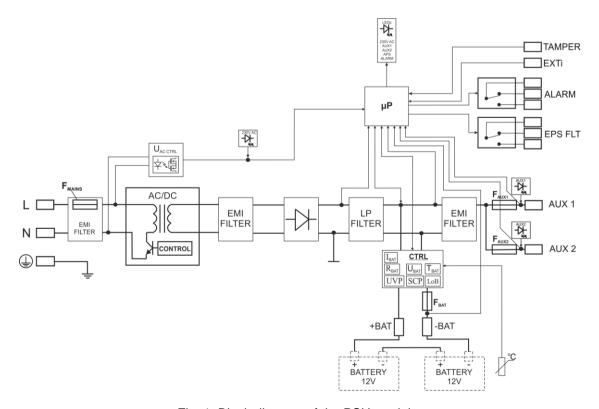
Fig. 1. Block diagram of the PSU module.
