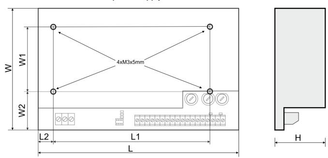
Fig. 3. Dimensions of power supply module.
